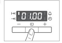
2. Using the End time → function, set the time at which the dish should be ready.
